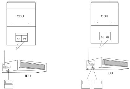
Fig. 4.7.3 One wired controller controls one IDU Fig. 4.7.4 Two wired controllers control one IDU
