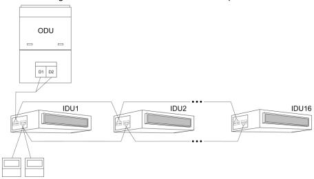
Fig. 4.7.6 Two wired controllers control multiple IDUs
