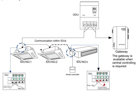
Fig. 4.7.1 Connection of single unit
