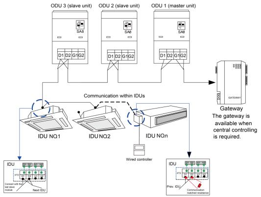
Fig. 4.7.2 Connection of modular units
