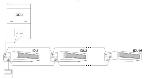
Fig. 4.7.5 One wired controller controls multiple IDUs
